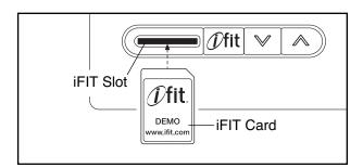
Next, select the desired workout on the iFIT card by pressing the up and down buttons next to the iFIT slot.
